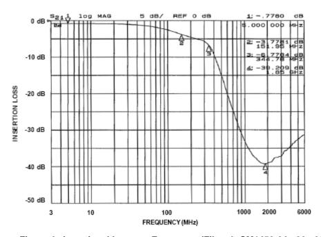
Figure 4. Insertional Loss vs. Frequency (Filter 4: CM1452-04, -06, -08)
