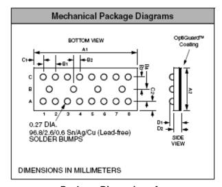
Package Dimensions for CM1452-08CP Chip Scale Package
