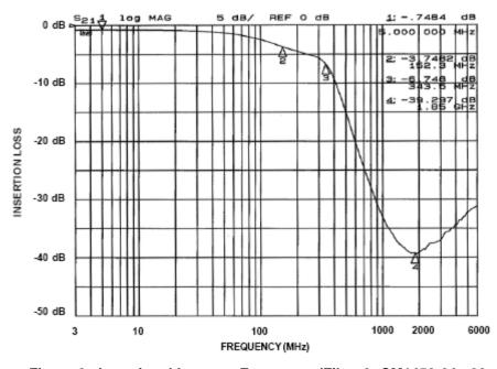
Figure 2. Insertional Loss vs. Frequency (Filter 2: CM1452-04, -06, -08)
