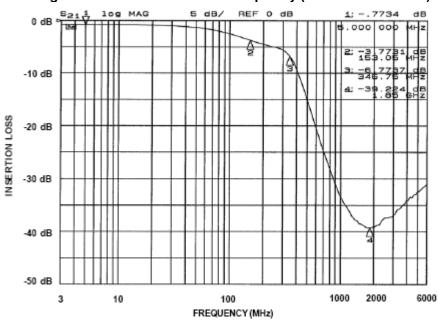
Figure 8. Insertional Loss vs. Frequency (Filter 8: CM1452-08)
