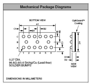
Package Dimensions for CM1452-06CP Chip Scale Package
