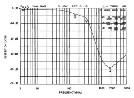
Figure 3. Insertional Loss vs. Frequency (Filter 3: CM1452-04, -06, -08)
