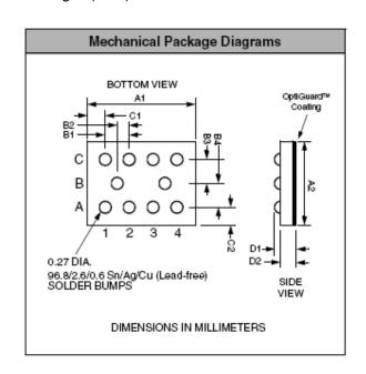
Package Dimensions for CM1452-04CP Chip Scale Package
