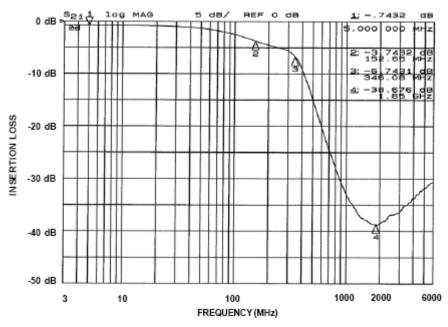
Figure 6. Insertional Loss vs. Frequency (Filter 6: CM1452-06, -08)
