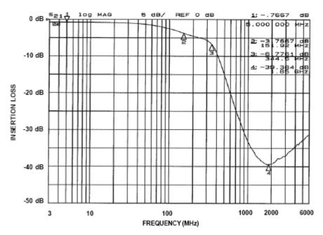
Figure 5. Insertional Loss vs. Frequency (Filter 5: CM1452-06, -08)
