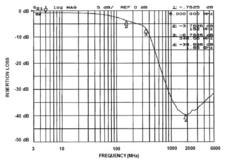
Figure 7. Insertional Loss vs. Frequency (Filter 7: CM1452-08)
