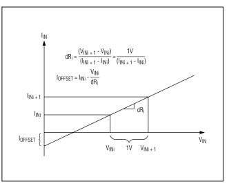
Figure 2. Effective Differential Resistance and Offset Current
