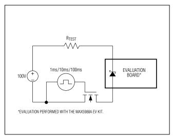
Figure 1. MAX5991A/MAX5991B Internal TVS Test Setup
