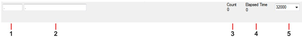
1. Text entered here is appended to the default file name and stored in the log file. The file name contains the Part Name and address shown in the large "Gesture Sensor" window, an underscore "\_" and the text entered. The default, if nothing is entered, is a period (".").
