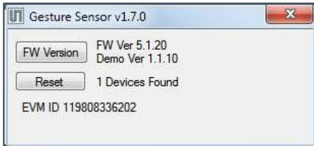
The Child Window contains the user interface with control buttons, fields, selection boxes and output values for the identified device connected. Tabs are used to make control and evaluation of specific device functions easy. For the TMG4903 device the initial display screen is shown:
