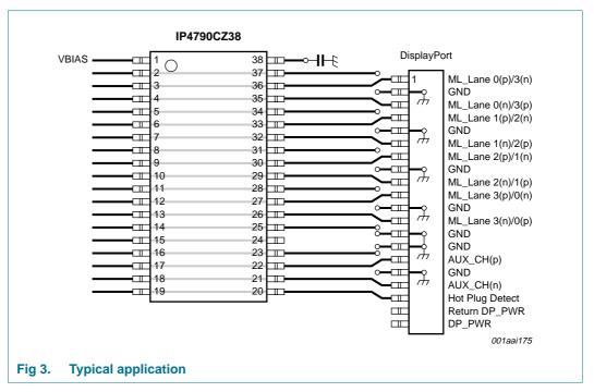
Connecting an optional 100 nF capacitor to the BIAS\_CAP pin (lead 38) enhances the ESD protection clamping performance. The VBIAS pin reduces the capacitive load of the ESD protection and  $V_{VBIAS}$  can be in the range 2.5 V to 5.5 V.
