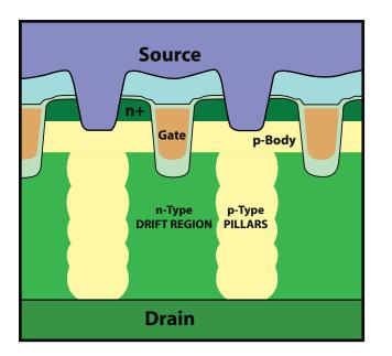
NextPower uses an optimized balance of the different resistance elements in the MOSFET to achieve a lower on-resistance for every cell. The low cell resistance means that NextPower types typically require fewer cells than competitor devices to achieve the same  $R_{DS(on)}$ , and a lower cell count provides lower  $Q_{G(tot)}$ , low  $Q_{GD}$ , low  $C_{oss}$  and superior 'Safe operating area' ruggedness.
