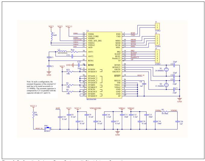
Figure 9. Configuration for Lower Power Systems with Direct Antenna Connections
