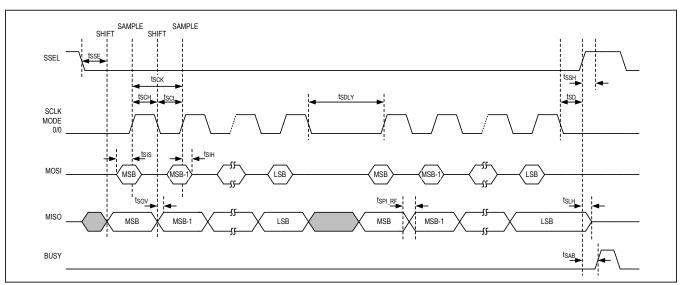
Figure 6. SPI Timing Specification
