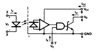
Note enable pin 7. An external 0.01  $\mu F$  to 0.1  $\mu F$  bypass capacitor must be connected between  $V_{CC}$  and ground for each package type.
