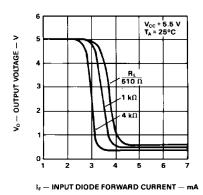
Figure 3 Input Diode Forward Characteristics
