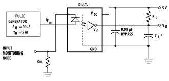
\* C  $_{\rm L}$  includes probe and stray wiring capacitance.
