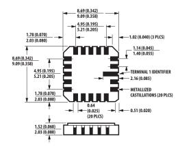
NOTE: DIMENSIONS IN MILLIMETERS (INCHES). SOLDER THICKNESS 0.127 (0.005) MAX.
