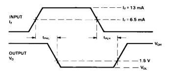
Figure 5 Propagation Delay,  $t_{PHL}$  and  $t_{PLH}$  vs. Pulse Input Current,  $I_{FH}$
