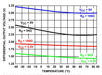
FIGURE 13. DRIVER DIFFERENTIAL OUTPUT VOLTAGE vs **TEMPERATURE**
