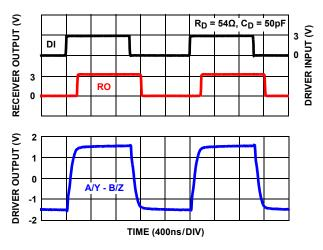
FIGURE 28.  $V_{CC}$  = 3.3V, DRIVER AND RECEIVER WAVEFORMS (ISL32453E, ISL32455E)
