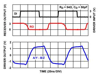
FIGURE 29.  $V_{CC}$  = 3.3V, DRIVER AND RECEIVER WAVEFORMS (ISL32458E, ISL32459E)
