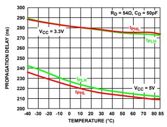
FIGURE 18. DRIVER DIFFERENTIAL PROPAGATION DELAY vs **TEMPERATURE (ISL32450E, ISL32452E, ISL32457E)**
