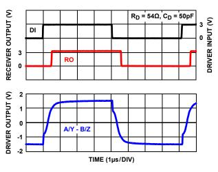
FIGURE 27. V<sub>CC</sub> = 3.3V, DRIVER AND RECEIVER WAVEFORMS (ISL32450E, ISL32452E, ISL32457E)
