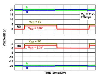
FIGURE 26. ±20V RECEIVER PERFORMANCE (ISL32458E, ISL32459E)
