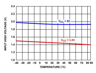
FIGURE 33. LOGIC INPUT HIGH VOLTAGE vs TEMPERATURE
