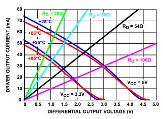
FIGURE 12. DRIVER OUTPUT CURRENT vs DIFFERENTIAL OUTPUT VOLTAGE
