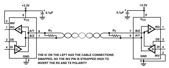
FIGURE 5. ISL32457E, ISL32459E HALF DUPLEX NETWORK USING CABLE INVERT FUNCTION
