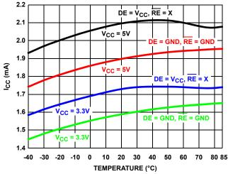
FIGURE 14. SUPPLY CURRENT vs TEMPERATURE
