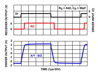
FIGURE 30. V<sub>CC</sub> = 5V, DRIVER AND RECEIVER WAVEFORMS (ISL32450E, ISL32452E, ISL32457E)
