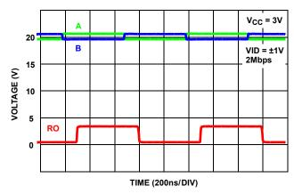
FIGURE 1. EXCEPTIONAL ISL32453E RX OPERATES AT >1Mbps EVEN WITH ±20V COMMON-MODE VOLTAGE
