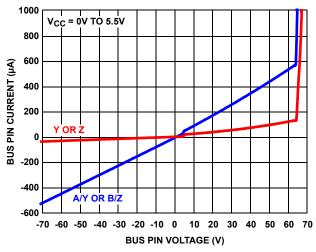
FIGURE 16. BUS PIN CURRENT vs BUS PIN VOLTAGE
