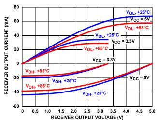
FIGURE 15. RECEIVER OUTPUT CURRENT vs RECEIVER OUTPUT **VOLTAGE**
