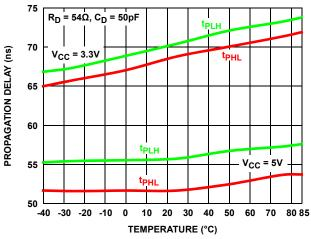
FIGURE 20. DRIVER DIFFERENTIAL PROPAGATION DELAY vs TEMPERATURE (ISL32453E, ISL32455E)
