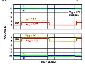
FIGURE 24. ±20V RECEIVER PERFORMANCE (ISL32450E, ISL32452E, ISL32457E)
