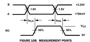
FIGURE 10. RECEIVER PROPAGATION DELAY AND DATA RATE
