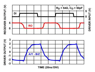
FIGURE 32.  $V_{CC}$  = 5V, DRIVER AND RECEIVER WAVEFORMS (ISL32458E, ISL32459E)
