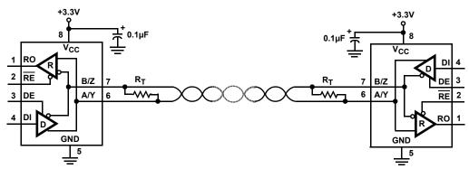
FIGURE 4. ISL32452E, ISL32455E, ISL32458E HALF DUPLEX NETWORK
