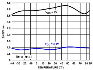
FIGURE 21. DRIVER DIFFERENTIAL SKEW vs TEMPERATURE (ISL32453E, ISL32455E)
