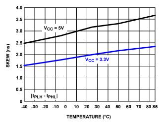
FIGURE 23. DRIVER DIFFERENTIAL SKEW vs TEMPERATURE (ISL32458E, ISL32459E)
