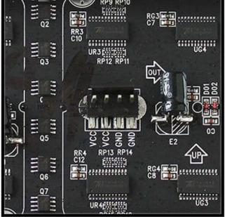
On the left is a screw post power connector (with adjacent pads for soldering wires directly). On the right, a Molex-style header. Some panels will have *two* headers...the power cable included with these panels has connectors for both headers.
