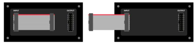
A dual-row header gets installed on the proto shield, similar to the connector on the matrix. Just like the ribbon cable lying flat, as long as these two headers are *aligned the same way*, they'll **match pin-for-pin**; unlike the jumper wire method from the prior page, mirroring doesn't happen.
