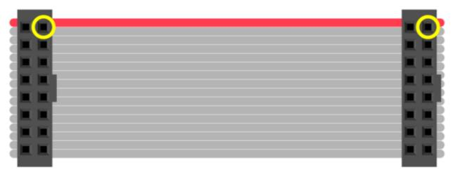
Plugged into a socket on the LED matrix, one header now faces *away* from you. If you double the cable back on itself (not a twist, but a fold)...to access a specific pin on the socket, the left and right columns are now mirrored (rows are in the same order — the red stripe provides a point of reference). You're looking "up" into the plug rather than "down" into the socket.
