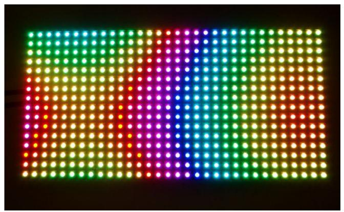
Of course, we wouldn't leave you with a datasheet and a "good luck!" We have a full wiring diagrams and working Arduino library code with examples from drawing pixels, lines, rectangles, circles and text. You'll get your color blasting within the hour! On an Arduino Uno or Mega, you'll need 12 digital pins, and about 800 bytes of RAM to hold the 12-bit color image (double that for the 32x32 matrix).
