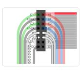
Pins A, B, C and D select which two rows of the display are currently lit. (32x16 matrices don't have a "D" pin — it's connected to ground instead.)
