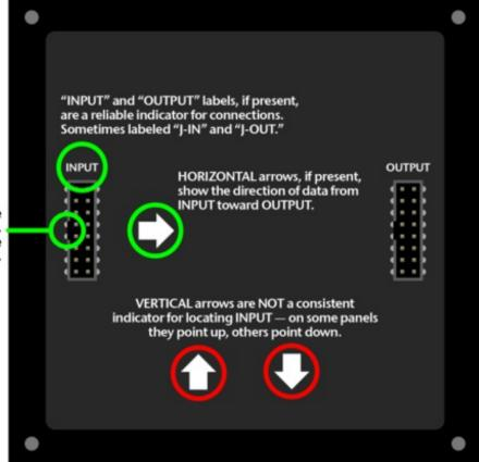
If there are no labels of any kind, the notch in the header shroud is a hint. On the INPUT connector, it faces the outer edge of the panel, not the center.
