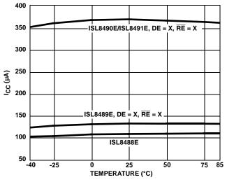
FIGURE 9. SUPPLY CURRENT vs TEMPERATURE
