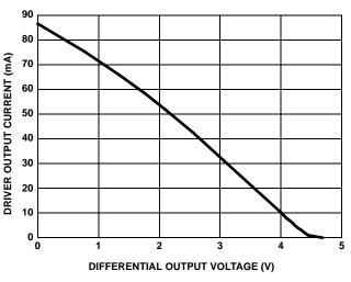
FIGURE 6. DRIVER OUTPUT CURRENT vs DIFFERENTIAL **OUTPUT VOLTAGE**
