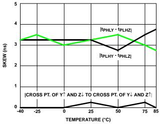
FIGURE 13. DRIVER SKEW vs TEMPERATURE (ISL8490E/ISL8491E)
