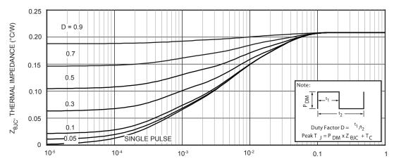
RECTANGULAR PULSE DURATION (SECONDS) Figure 1, Maximum Effective Transient Thermal Impedance, Junction-To-Case vs Pulse Duration
