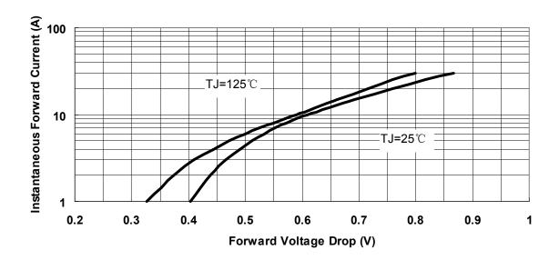
Fig.3-Typical Instantaneous Forward Voltage Characteristics
