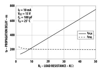
Figure 9. Propagation Delay vs. Load Resistance.
