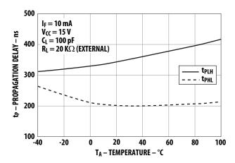
Figure 8. Propagation Delay with External 20  $k\Omega$  RL vs. Temperature.
