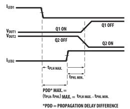
NOTE: THE PROPAGATION DELAYS USED TO CALCULATE PDD ARE TAKEN AT EQUAL TEMPERATURES.
