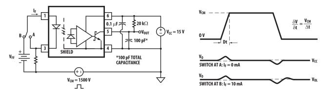
Figure 7. CMR Test Circuit.
