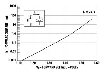
Figure 5. Input Current vs. Forward Voltage.
