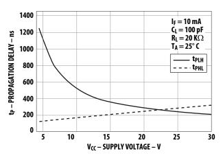
Figure 11. Propagation Delay vs. Supply Voltage.
