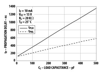
Figure 10. Propagation Delay vs. Load Capacitance.
