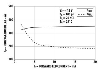
Figure 12. Propagation Delay vs. Input Current.
