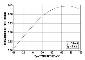
Figure 3. Normalized Output Current vs. Temperature.
