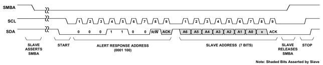
After OUT5/SMBA has been released, the bus master (typically a microcontroller) may opt to perform some service functions in which it may send data to or read data from the ispPAC-POWR1220AT8. As part of the service functions, the bus master will typically need to clear whatever condition initiated the SMBAlert request, and will also need to reset GP5\_ENb to re-enable the SMBAlert function. For further information on the SMBus, the user should consult the SMBus Standard.
