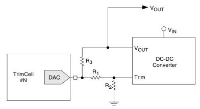
Figure 16 shows the resistor network between the TrimCell #N in the ispPAC-POWR1220AT8 and the DC-DC converter. The values of these resistors depend on the type of DC-DC converter used and its operating voltage range. The method to calculate the values of the resistors R1, R2, and R3 are described in a separate application note.
