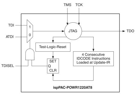
Table 12 shows in truth table form the same conditions required to select either TDI or ATDI as in the logic diagram found in Figure 36.
