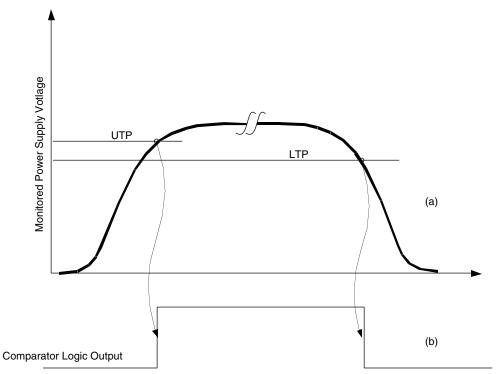
During power supply ramp-up the comparator output changes from logic 0 to 1 when the power supply voltage crosses the upper trip point (UTP). During ramp down the comparator output changes from logic state 1 to 0 when the power supply voltage crosses the lower trip point (LTP). To monitor for over voltage fault conditions, the UTP should be used. To monitor under-voltage fault conditions, the LTP should be used.
