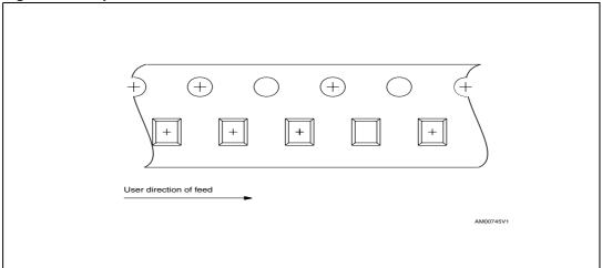
1. Pin A1 is at top left corner based on above tape orientation.
