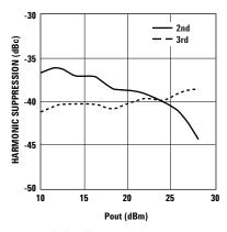
Figure 8. 2nd/3rd Harmonics vs. Pout.
