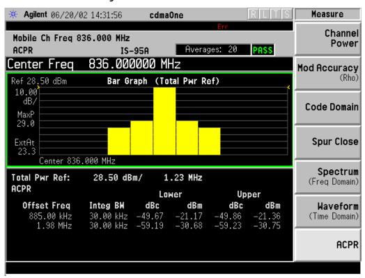
Figure 18. ACPR measurement using VSA Transmitter tester.
