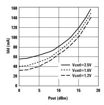
Figure 5. Idd vs. Output Power.
