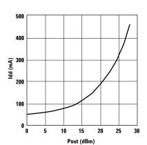
Figure 4. Idd vs. Output Power.
