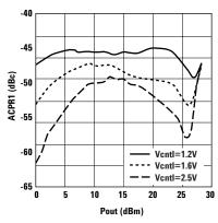
Figure 6. ACPR (1.25 MHz offset) vs. Pout.
