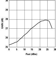
Figure 9. Gain vs. Pout.
