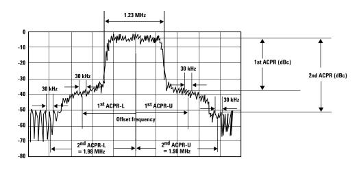
Figure 16. CDMA Adjacent-Channel Power Ratio Measurement.
