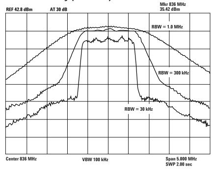
Figure 19. Example ACPR measurement using Spectrum Analyzer.
