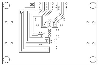
Figure 23. Layer 3 - Bottom Metal & Solder Mask.
