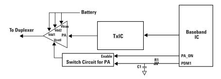
If PDM1 can be controlled then same circuit can be used for Dynamic bias control
