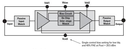
Figure 24. Power Module Block Diagram.
