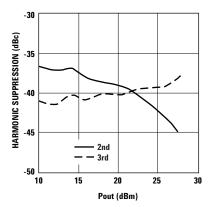
Figure 14. Harmonic Suppression vs. Pout.
