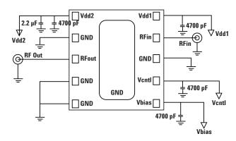
Figure 20. ACPM-7833 Evaluation Board Schematic and Layout.
