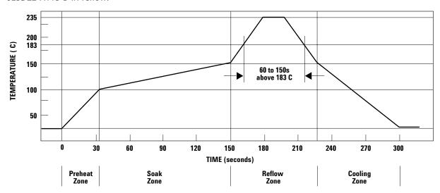
Figure 25. Time-temperature Profile for IR Reflow Soldering Process.
