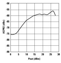
Figure 13. ACPR (1.98 MHz offset) vs. Pout.
