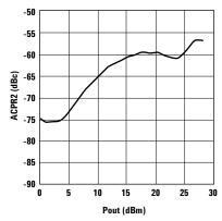
Figure 7. ACPR (1.98 MHz offset) vs. Pout.
