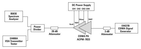
Figure 17. ACPR test equipment setup.
