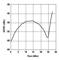
Figure 12. ACPR (1.25 MHz offset) vs. Pout.
