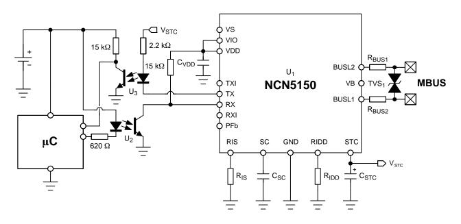
Figure 6. Optically Isolated Application Schematic
