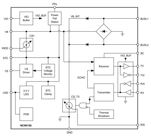
Figure 2. NCN5150 Block Diagram
