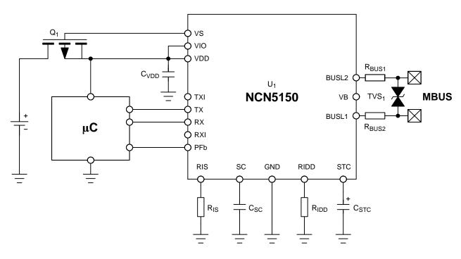
Figure 5. Application Schematic with Backup External Power Supply
