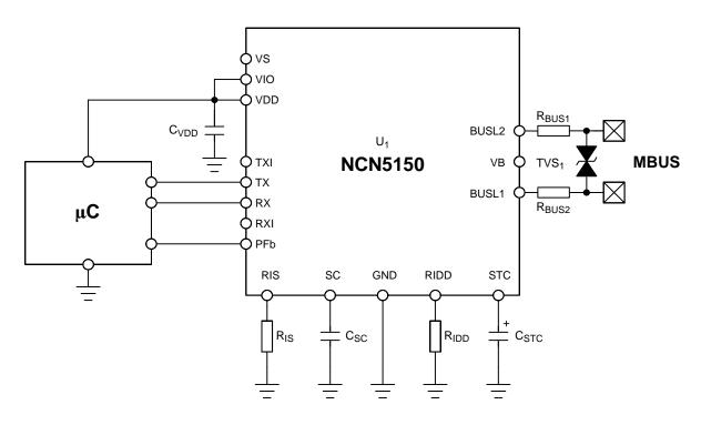
Figure 3. General Application Schematic
