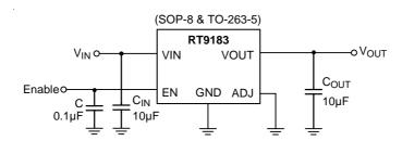
Figure 3. Fixed Operation with SOP-8 and TO-263-5 packages
