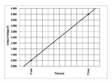
OUTPUT VOLTAGE =  $\frac{80\% \times \text{Supply V}}{\text{Pmax-Pmin}} \times \{\text{Pressure applied -Pmin}\} + 0.500$
