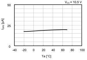
Current consumption vs. temperature in power-down mode
