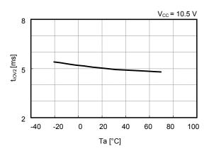
Overcurrent 3 (load short) detection time vs. temperature
