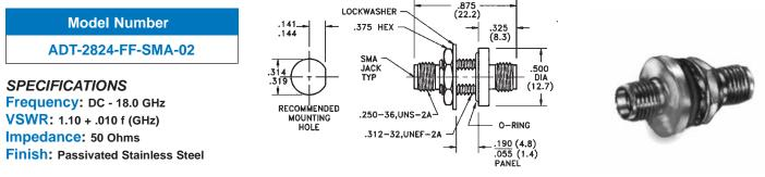
Standard finish is passivated stainless steel, for gold plating change -02 suffix to -00.
