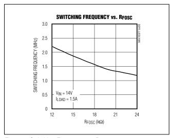
Figure 2. Switching Frequency vs. R<sub>FOSC</sub>
