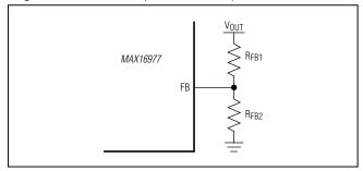
Figure 1. Adjustable Output-Voltage Setting
