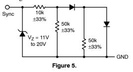
The rising edge of the sync pulse turns on the power switch to start a new switching cycle, as shown in Figure 6. There is approximately 0.5  $\mu s$  delay between the rising edge of the sync pulse and rising edge of the  $V_{SW}$  pin voltage. The sync threshold is TTL logic compatible, and duty cycle of the sync pulses can vary from 10% to 90%. The frequency foldback feature is disabled during the sync mode.
