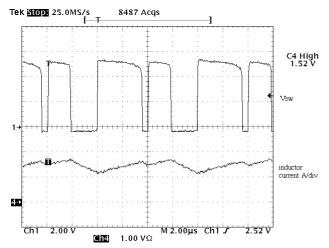
Figure 8. The Regulator in Current Limit
