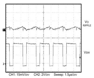
Figure 16. Output Voltage Ripple Using One 100  $\mu$ F POSCAP Capacitor
