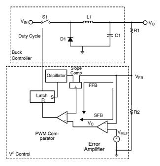
Figure 3. Buck Converter with V<sup>2</sup> Control.
