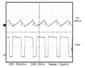
Figure 18. Output Voltage Ripple Using One 100 μF Tantalum Capacitor
