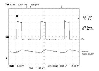
Figure 12. In Short Circuit, the Foldback Current and Foldback Frequency Limit the Switching Current to Protect the IC, Inductor and Catch Diode
