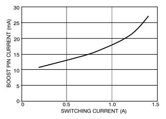
Figure 9. The Boost Pin Current Includes 7.0 mA
