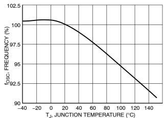
Figure 4. Oscillator Frequency Versus Junction Temperature
