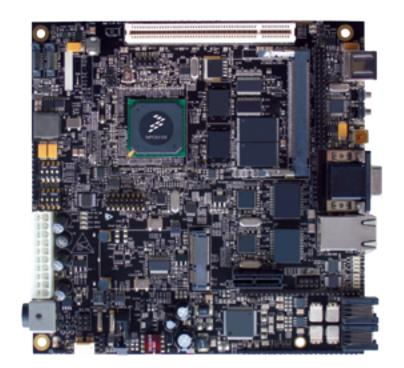
A board support package (BSP) is pre-installed on the MPC8315E-RDB. This BSP includes a bootloader (u-boot)—a generic Power Architecture technology system based on the Linux<sup>®</sup> kernel. The u-boot and Linux kernel reside in the on-board flash memory.
