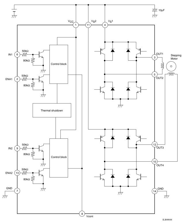
\* There are no constraints on the relationship between the applied voltage to  $V_{CC}$ ,  $V_{S1}$ ,  $V_{S2}$ , ENA1, ENA2, IN1, and IN2 within the absolute maximum ratings (For example, this IC can be used at  $V_{CC}=3V$ ,  $V_{S1}=V_{S2}=2V$ , and ENA=IN=5V)
