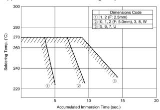
Perform soldering within tolerance range (shaded portion).
