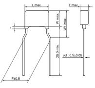
Coating extension does not exceed the end of the lead bend Lead Wire: Solder Coated Copper Wire or Solder Coated CP Wire (ir (in mm)
