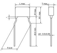
Coating extension does not exceed the end of the lead bend. Lead Wire : Solder Coated Copper Wire or Solder Coated CP Wire
