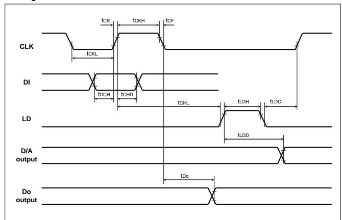
(Note) Timing chart above is a schematic representation of the timing of each signal type. CLK signal input is High or Low regardless, LD signal High input is enabled.
