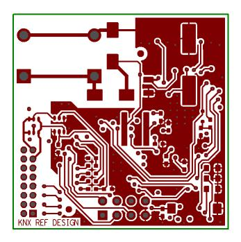
Figure 11. Top Layer of NCN5120 Reference Design
