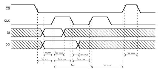
Figure 6. SPI Bus Timing Diagram
