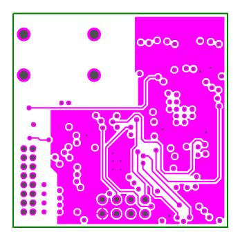
Figure 13. Inner Layer 1 of NCN5120 Reference Design
