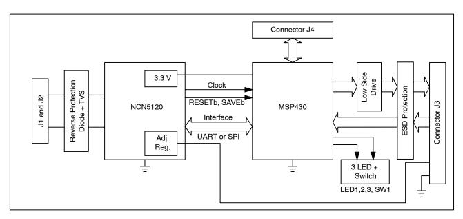
Figure 2. NCN5120 Reference Design Block Diagram
