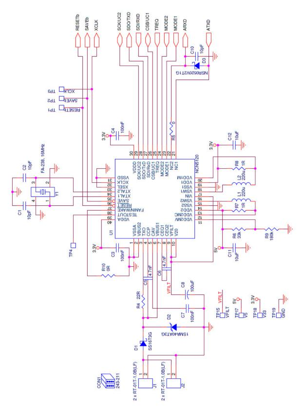
Figure 9. Schematic of NCN5120 Reference Design (Part 1)
