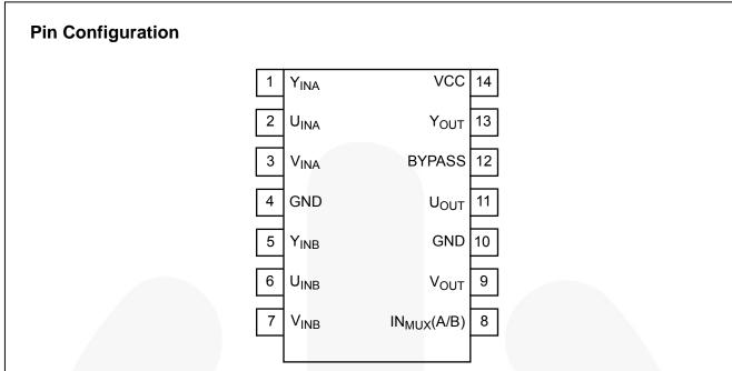
Figure 2. Pin Configuration
