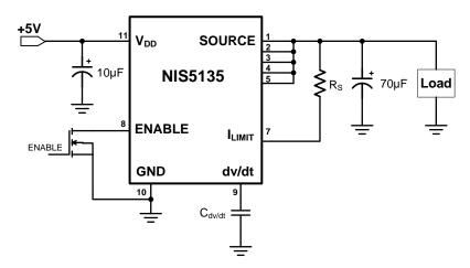
Figure 1. Application Circuit with Direct Current Sensing
