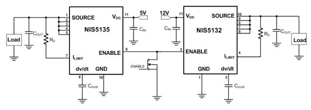
Figure 3. Application Circuit with Common Thermal Shutdown
