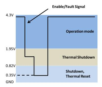
Figure 4. Enable/Fault Signal Levels
