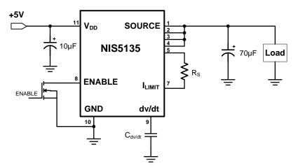
Figure 2. Application Circuit with Kelvin Current Sensing
