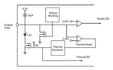
**Enable/Fault Function Circuit**
